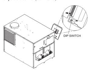
FIG. 49 User Access Level Dip Switch Location
